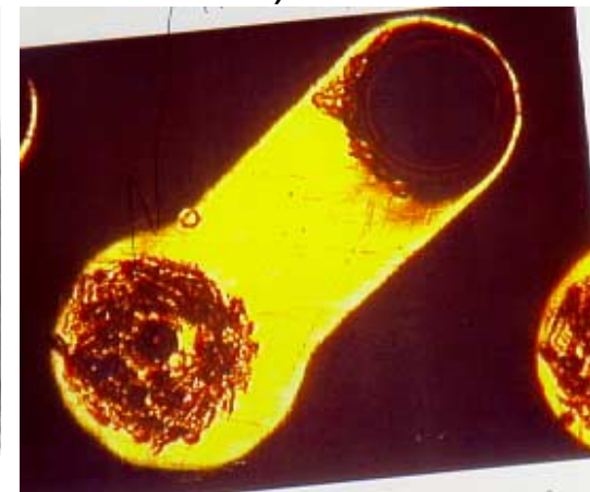
Fig 9. Inner pad damaged by pogo pin
